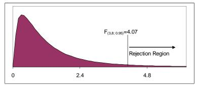
If the calculated F is larger than 4.07, we reject  $H_0$ : The treatments means are likely different, unless a 5% error has occurred.
